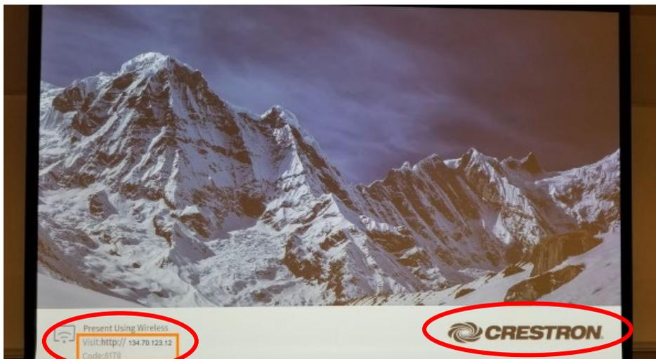
3. Open the Crestron AirMedia app and type in the numbers from the URL on the Crestron screen (no http:// needed, just the numbers). For example: 10.15.54.30. Press Enter to search for the server.
